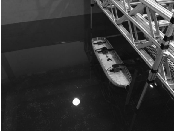
Figure 3: Setting model for a drift test in beam seas
